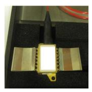
1. While the metal clip is still on the LD, pull it by a few mm from the LD case.
