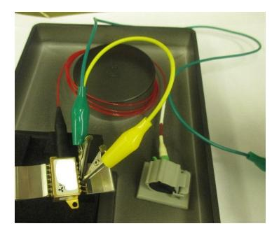
3. While the wire clip is still in place (or the short wire soldered) cut the pins of the LD to 7-8 mm from case and remove the original metal clips.
