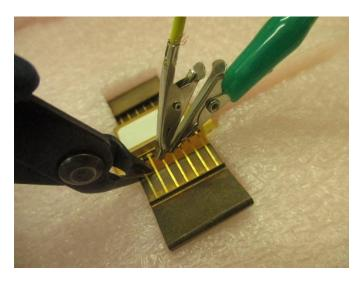
4. Apply a small amount of thermal grease on the LD bottom surface where it should connect to the heat sink.
